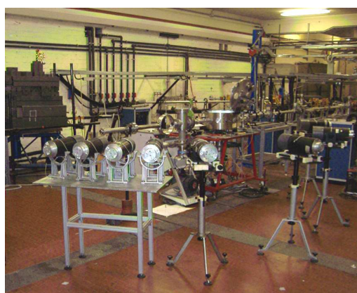
Figure 4: The ^8\text{B} experiment. 8 Photo Multiplier Tubes cover neutron angles from 15^\circ to 140^\circ in the lab frame.
