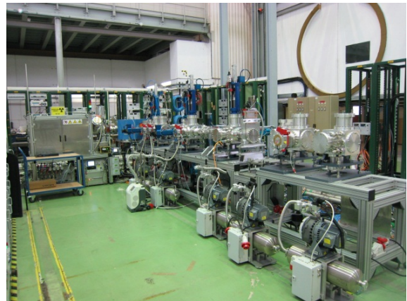
Figure 3: The MedAustron ITS at CERN, currently consisting of an ECR ion source, a spectrometer magnet and several different beam diagnostic tanks
