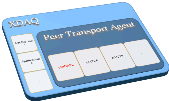
Fig. 12. ptuDAPL integration with XDAQ framework.
