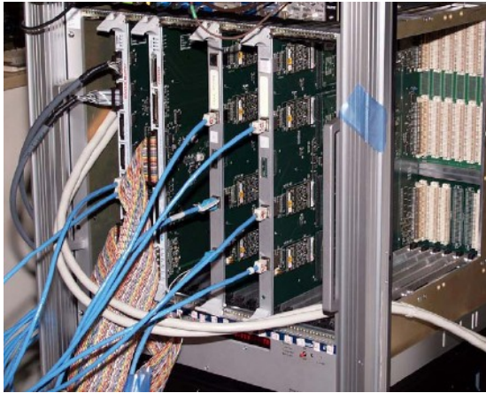
Figure 11: Picture of the VME crate housing the DAQ boards: NECO, Buffer and two FADC boards.
