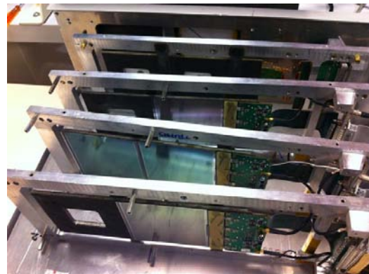
Figure 5: Telescope test sensors equipped with VAI chip and SiLC sensors.
