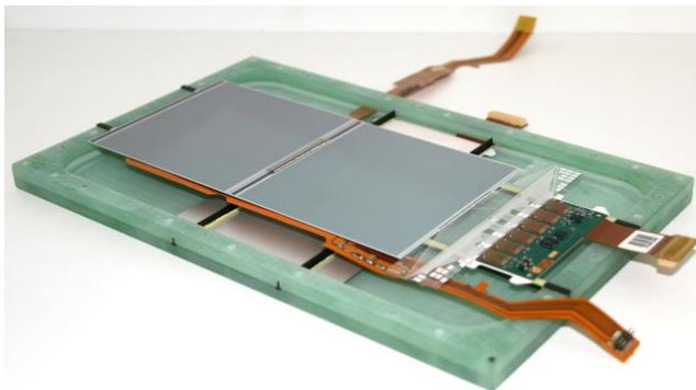
Figure 4: LPTPC modules equipped with SiLC sensors.
