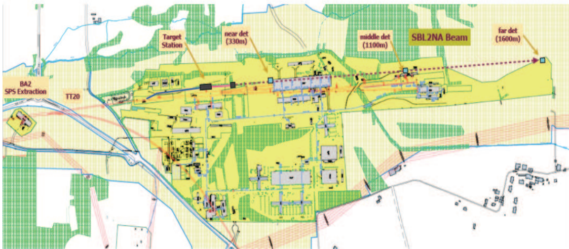
Figure 139. The new SPS North Area neutrino beam layout. Main parameters are: primary beam: 100 GeV; fast extracted from SPS; target station next to TCC2, \sim 11 m underground; decay pipe: 100 m, 3 m diameter; beam dump: 15 m of Fe with graphite core, followed by muon stations; neutrino beam angle: pointing upwards; at \sim 3 m in the far detector \sim 5 mrad slope.
