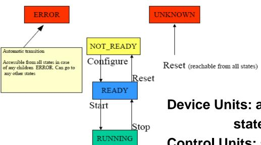
Further abstraction as finite state machines (SMI++): defined transition from one state of the board into another with possibility to autorecover
