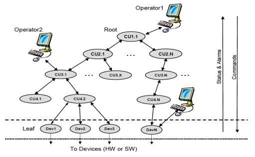
Extended to allow for finite state modeling & hierarchical control:
