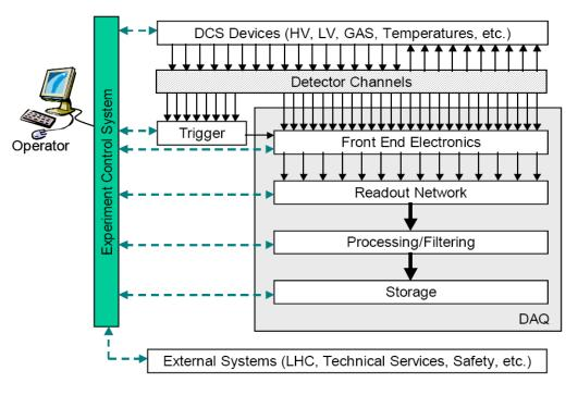
Configuration, monitoring and operation of the 'whole' experiment:
