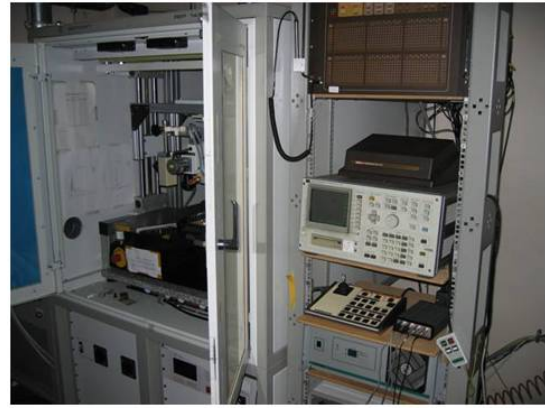
Figure 4. X-ray test setup for single transistor devices, comprising a HP4145 and a Keithley 707.
