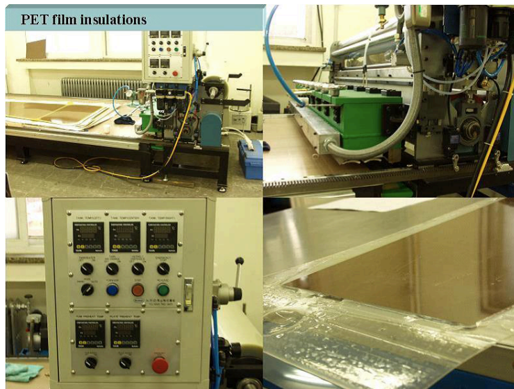
Figure 5: The graphite layer of the electrode is covered with the Mylar film for the protection.
