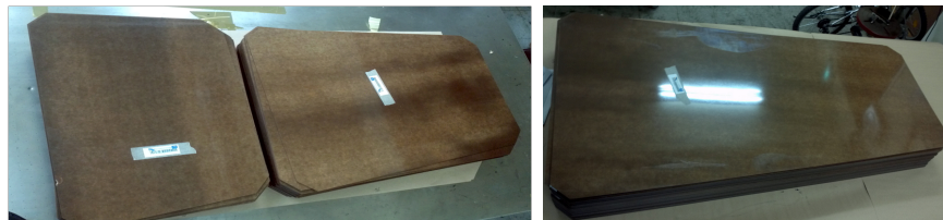
Figure 3: Bakelites are cut for RE4/2 top narrow and top wide gaps (left), and bottom gaps (right).
