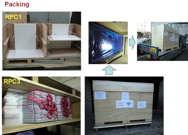
Figure 9: Qualified gas gaps being loaded in a specially designed box. The extra space to absorb any impact on the box is shown near the bottom of the photo.
