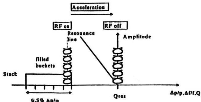
The beam is trapped in small buckets created at the top of the stack.
