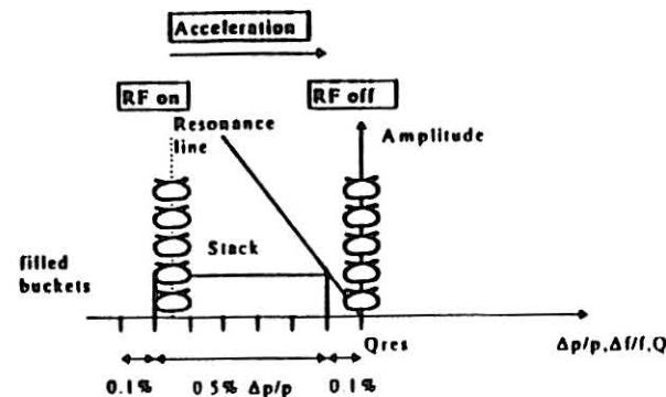
The beam is trapped in small buckets created at the bottom of the stack.
