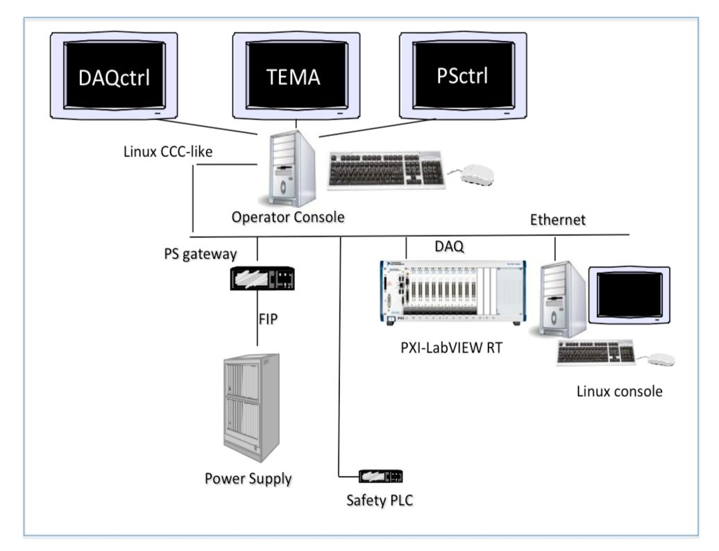
The first step of the upgrade of the Measurement Systems was to replace the existing VME based Data Acquisition (DAQ) system with a new one based on PXI hardware and LabVIEW RT.
