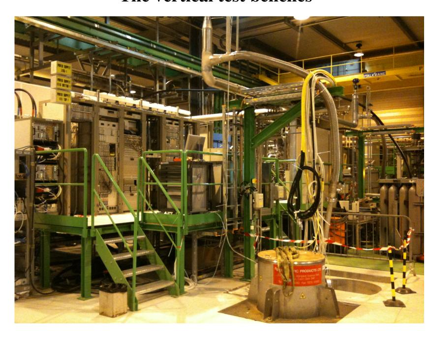
The vertical test station is now equipped with 4 cryostats of different dimensions for different purposes: 3 of them were used in the previous facility and a 4th, the biggest, is procured within the High Field Magnet (HFM) project for the FRESCA2 magnet.
