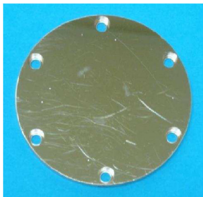
FIG. 51. Glidcop® pulsed heating sample after the 110°C test. The scratches on the surface occurred prior to testing the sample.
