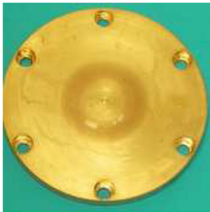
FIG. 29. Photograph of electrodeposited copper sample after processing up to a pulsed heating temperature of 110°C.
