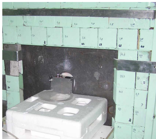
Fig. 1. Positioning of the RadMon detector in the BNCT beam line.
