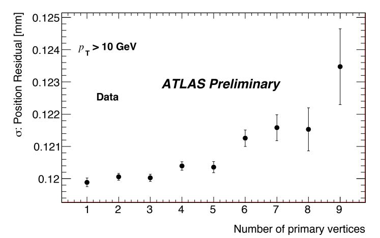
Position residual width (barrel+endcap) as a function of the number of reconstructed primary vertices found in the event
