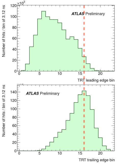
LHC currently running with 50 ns bunch spacing - easily handled by cutting on leading edges that are too large, and requiring valid 0->1 transition. Next year, may see 25 ns spacing!
