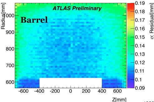
Position residual width as a function of R and Z in data for barrel (left) and endcap A (below). The widening of residuals at large Z and large radius is reproduced by the simulation
