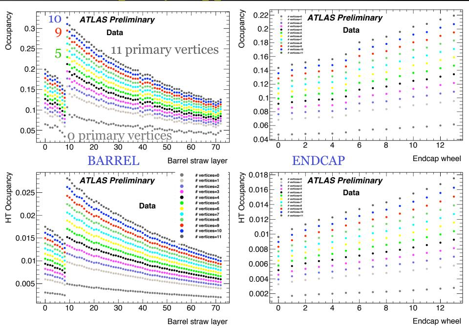
Look at how the occupancy changes as an additional reconstructed primary vertex is found in the event. Should be a measure of the additional in-time occupancy from every minimum bias interaction.
