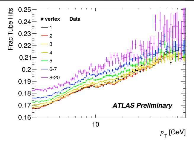
Fraction of TRT hits on track that are labeled as "non-precision hits" by the tracking software, as a function of track pt, shown for events with different numbers of reconstructed primary vertices
