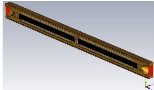
Figure 1: Jaw model of the mock-up collimator with in-jaw BPM buttons [7].
