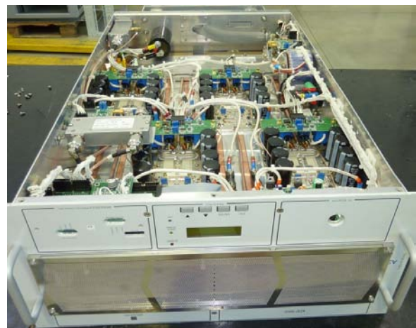
Figure 2: 7 kW amplifier unit
