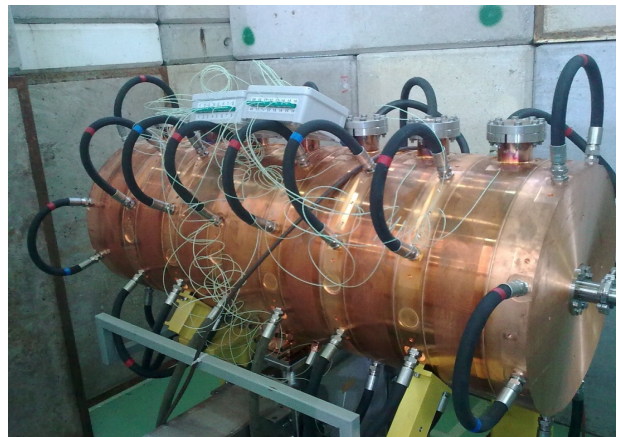
Figure 1: The PIMS cavity connected inside the bunker.
