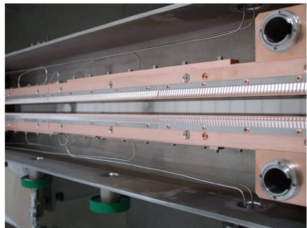
Figure 3: The two copper jaws and the special cables inside the collimator demonstrator (no upper tank cover).
