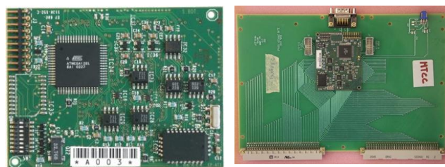
Figure 1: ELMB and PTHM electronic boards with ELMB.
