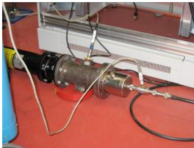
Figure 11: Calibration of the directional coupler by low level measurements.
