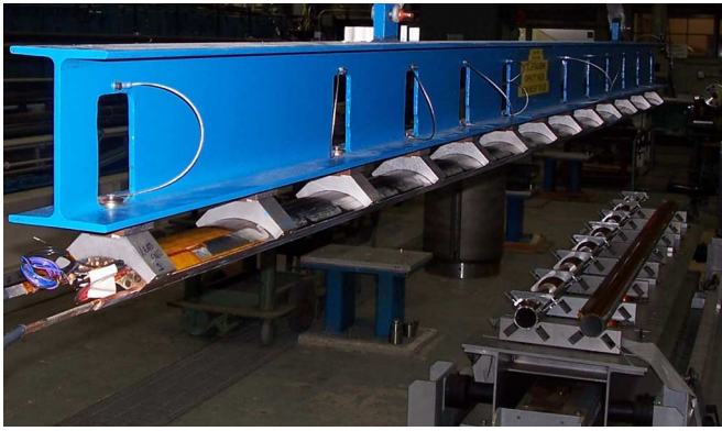
Fig. 2. LQ coil after impregnation being moved to the shipping mandrel.
