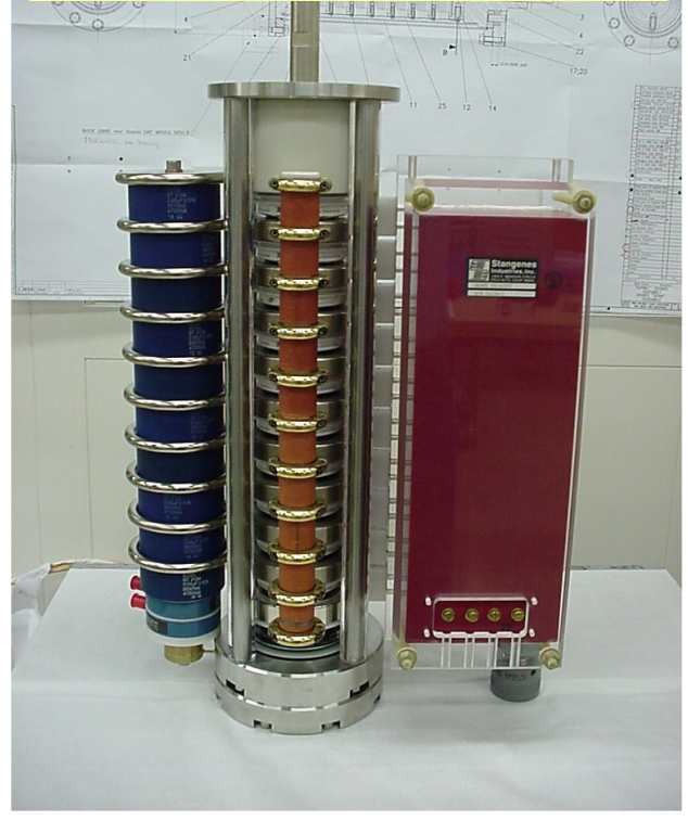
GTO stack with trigger transformer (right)
