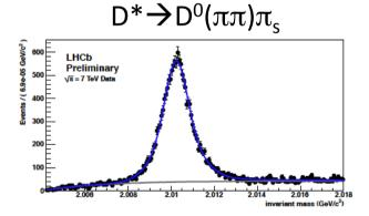
• Using world averages of the physical asymmetries we can solve the system of equations for the instrumental asymmetry  $A_D(K\pi)$
