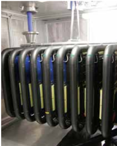
Figure 2.21 Left: SLAC P1 Marx modulator showing its cantilevered support structure, high-voltage grading rings, and 16 installed cells. Right: RF waveforms from one of the two klystron ports: no droop compensation (blue), with only delay cells (green), with delay cells and Vernier (red), producing a flat pulse with a 3% saw-tooth pattern.
