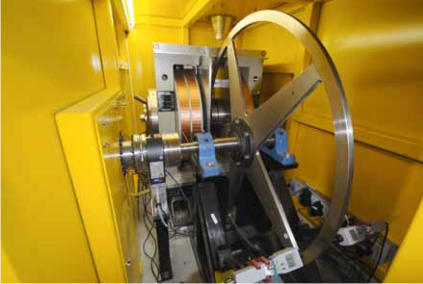
Figure 3.23 Prototype rotating target setup for eddy current tests at Daresbury Lab. Copyright STFC.
