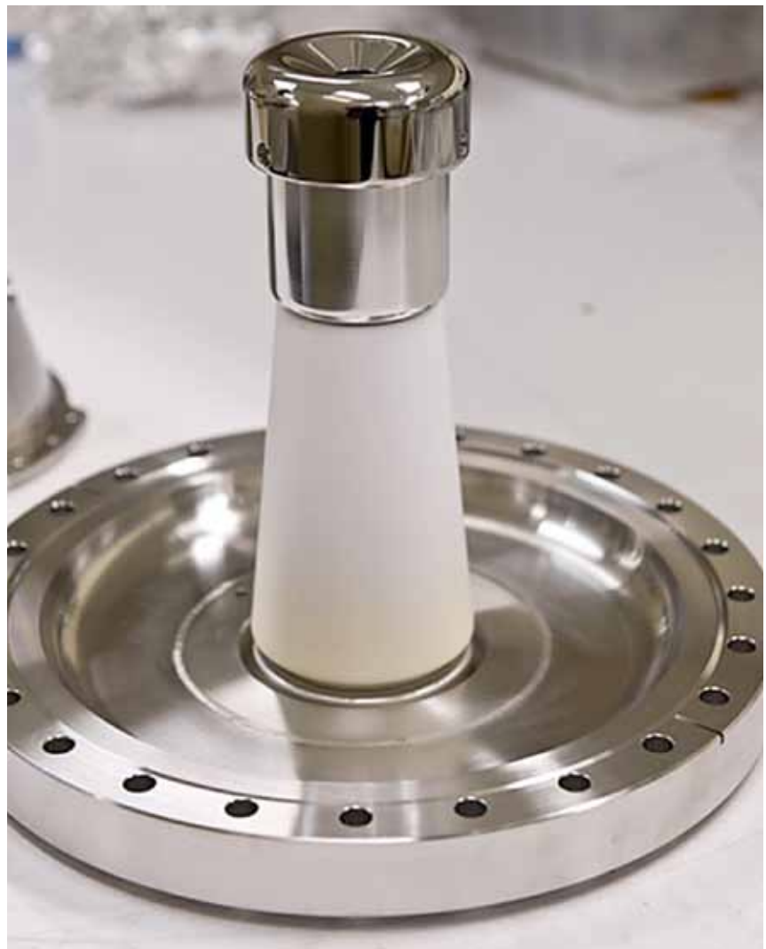
Figure 3.20 Niobium electrode of inverted gun design.
