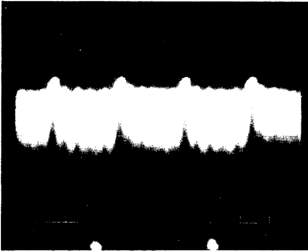
Fig. 5. Direct output of the photomultiplier. Scaling: vertical 5 mV/div.; horizontal 10 \mu s/div.
