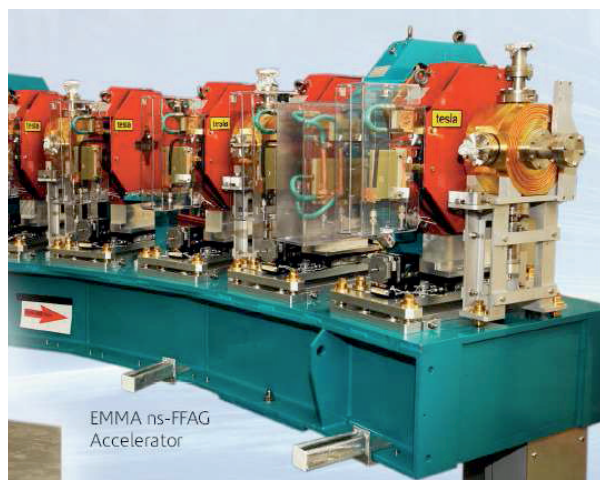
Fig. 5: EMMA accelerator components installed on a girder.
