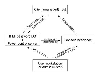
Figure 1. Communication diagram of the system components
