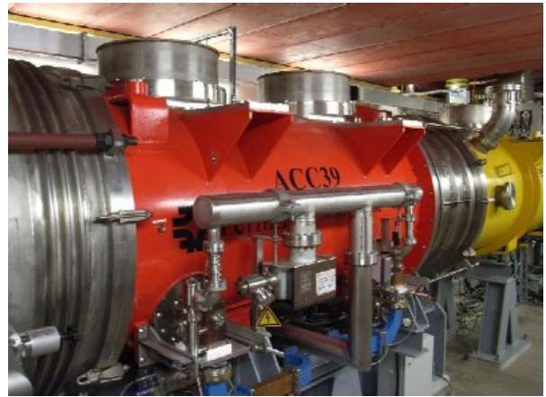
Figure 1: ACC39 module in FLASH beam line. ACC1 can be seen in yellow at the right of the picture.
