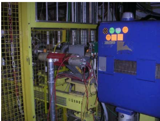
Figure 11 BLM 3: (SPS-Position: 51910) seen from the inside of the machine (left) and from top (right). It is installed close to the corrector MDV.51910 and to the corresponding SPS BLM (installed closer to the beam pipe in the picture). It is placed parallel to the beam pipe at a distance of 44 cm to the beam pipe wall. Courtesy of E. Effinger.
