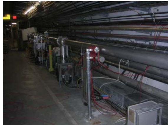
Figure 10 BLM 2 and SEM 2: (SPS-Position: 51956) seen from the inside of the machine (left) and from top (right). They are positioned 500 cm downstream of BLM6 (see below). The BLM and SEM are installed parallel to the beam pipe at a distance of 3 cm to the beam pipe wall. The SEM is centred vertically and the BLM 15 cm lower. Courtesy of E. Effinger.
