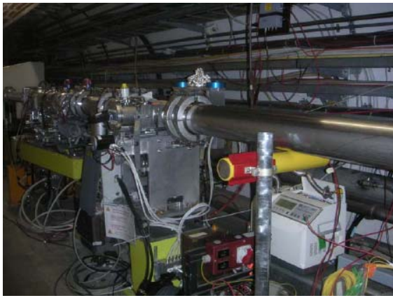
Figure 13 BLM 6: (SPS-Position: 51938) seen from the inside of the machine (left) and from top (right) Distance: 100 cm from middle of the Roman Pot 1 to the BLM. It is placed perpendicular to the beam pipe at a distance of 2 cm to the beam pipe wall. Courtesy of E. Effinger.
