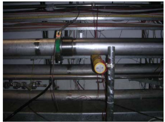
Figure 14 BLM 7: (SPS-Position: 51992) seen from inside the machine (left) and from top (right). It is installed at a distance of 100 cm downstream of the middle of the Roman Pot 2 (not installed yet). It is placed perpendicular to the beam pipe at a distance of 2 cm to the beam pipe wall. Courtesy of E. Effinger.
