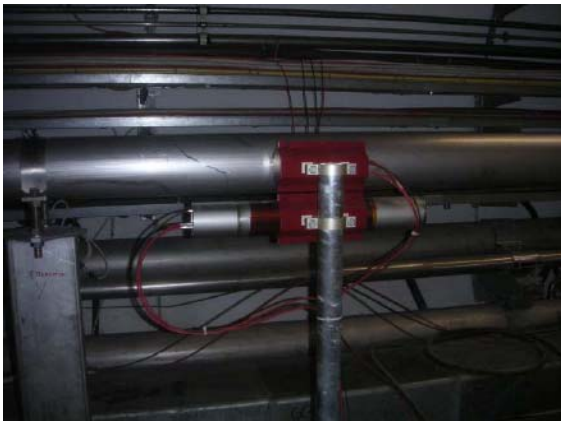
Figure 10 BLM 2 and SEM 2: (SPS-Position: 51956) seen from the inside of the machine (left) and from top (right). They are positioned 500 cm downstream of BLM6 (see below). The BLM and SEM are installed parallel to the beam pipe at a distance of 3 cm to the beam pipe wall. The SEM is centred vertically and the BLM 15 cm lower. Courtesy of E. Effinger.
