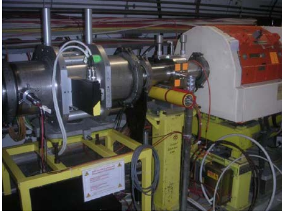
Figure 15 BLM 8: (SPS-Position: 51999) seen from the inside of the machine (left) and from top (right) at a distance of 67 cm downstream of the middle of TAL collimator (TACW.51998). It is placed perpendicular to the beam pipe at a distance of 1 cm to the beam pipe wall. Courtesy of E. Effinger.
