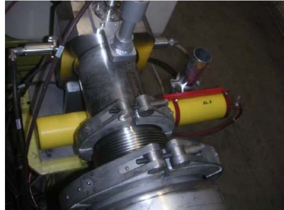
Figure 15 BLM 8: (SPS-Position: 51999) seen from the inside of the machine (left) and from top (right) at a distance of 67 cm downstream of the middle of TAL collimator (TACW.51998). It is placed perpendicular to the beam pipe at a distance of 1 cm to the beam pipe wall. Courtesy of E. Effinger.
