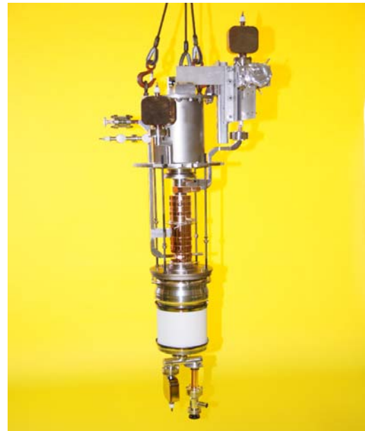
Figure 3: The XL5-1 klystron ready to ship.
