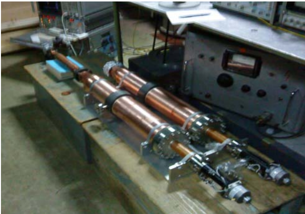
Figure 5: SLED-I type pulse compressor at cold testing
