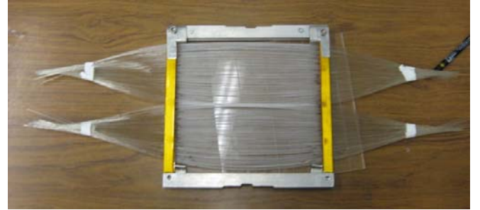
Fig. 12. The ribbon built with radiation hard WLS fiber prototype.
