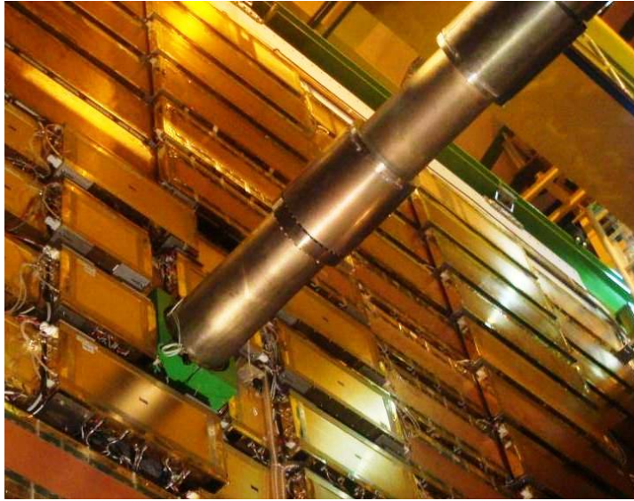
Figure 2.34: The fully mounted rectangular muon modules on one of the five muon stations in the beam pipe region. The transverse projective segmentation in the module dimensions can be seen, with a smaller modules mounted closer to the beam pipe to achieve a constant resolution across the whole detector plane.
