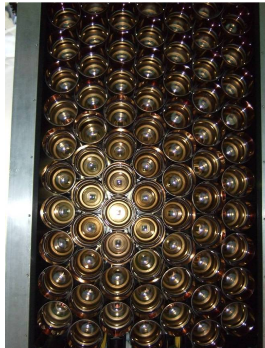
Figure 2.24: A photo of a complete HPD panel for the RICH1 showing the hexagonal arrangements of the HPDs.
