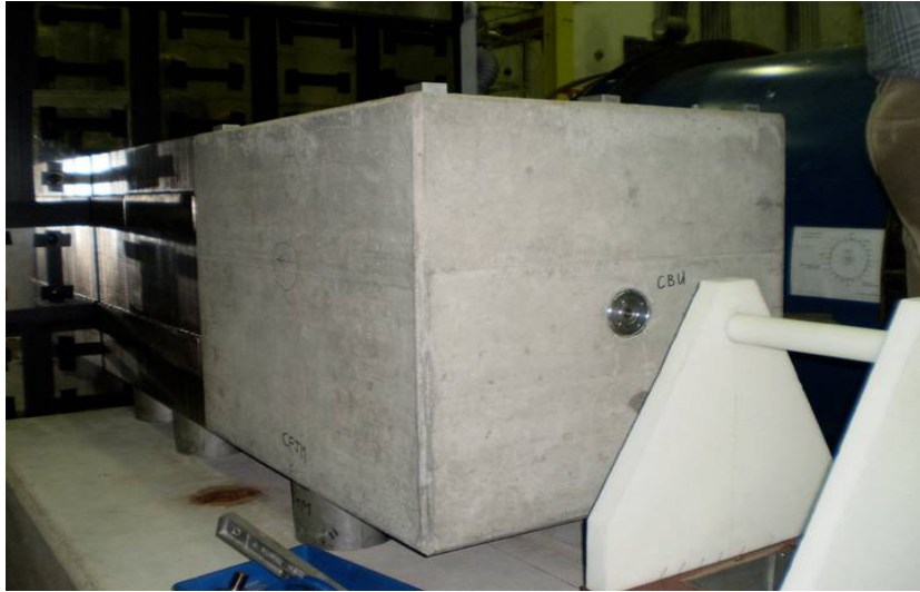
Figure 68: Photograph of the absorber and target setup for the 2009 beam test: on the right, inserted in two vertical supports, the two polyethylene target cells; on the left the concrete part of the absorber, with a section of the hollow aluminium cylinder filled with tungsten, followed by the stainless steel part on the very end of the picture. An additional concrete shielding was placed around the absorber to reduce the dose rate.
