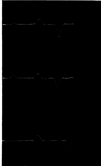
Fig. 3. Scope traces of the three counter pulses. The first is the pulse of P_2 , the second is that of the Čerenkov, the last that of P_1 . At left they are "good" and "bad" photon-proton pairs with proton recoils of (44.5 \pm 10\%) Mev. The good one is in the middle. At right the pulses are those due to photon-proton pairs with protons of (25 \pm 15\%) Mev.
