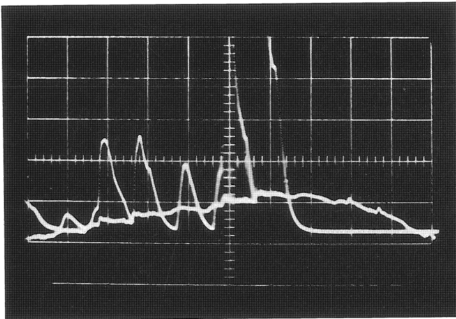
Fig. 17. The same as fig. 16 but at higher resolution, magnet ripple at 10 amp/cm. Sweep speed : 2 ms/cm. The coincidence between ripple and counter peaks is more easily seen.
