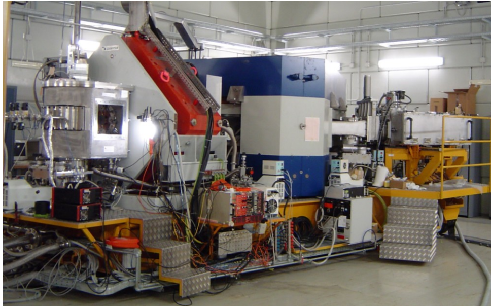
Fig.1: General view of the MAGNEX spectrometer. From the left to the right the scattering chamber, the quadrupole, the dipole and the Focal Plane Detector are visible.
