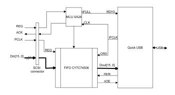
Figure 1: The block diagram of the Parallel to Serial Flow Converter (PSFC).
