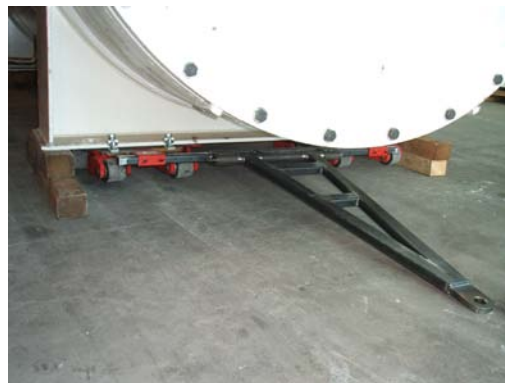
FIGURE 5. Cold box heavy load trolley
