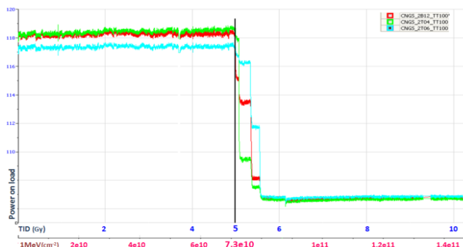
Figure 10: Three AC heater channels failing at the low dose station
