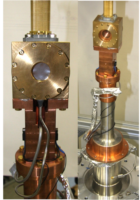
Figure 11: Photographs of the new cavity mounted on the coldhead.
