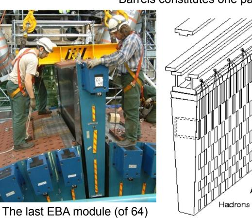
TileCal is a sampling calorimeter using iron as absorber and tiles of scintillating plastic as the active material. The tiles are oriented perpendicularly to the beam direction and staggered in radial depth. The light readout is done by WLS optical fibers, that couple to PMTs in the outer part of each module.
