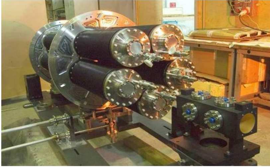
Figure 5. The CNGS target magazine consisting of five target units. The bottom unit intercepts the proton beam; the other four are in-situ spares.
