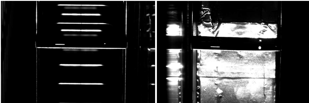
Figure 16. Pictures of a tray taken by the BMS vision system before (left) and after (right) insertion of bricks. The shadow of the tray visible on the brick surface is used to compute the distance of the brick with respect to the tray border.
