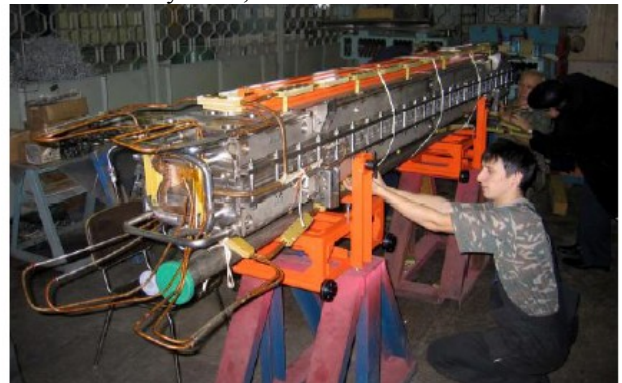
Figure 5: Curved, SIS100 full length dipole model after assembly at BINP
