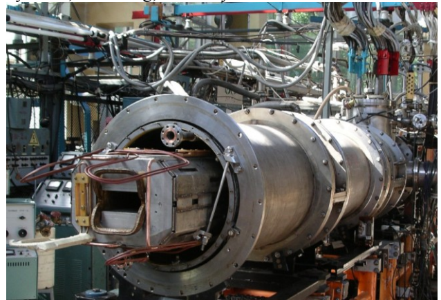
Figure 4: Full length, straight SIS100 model dipole at cold test built by JINR, Dubna
