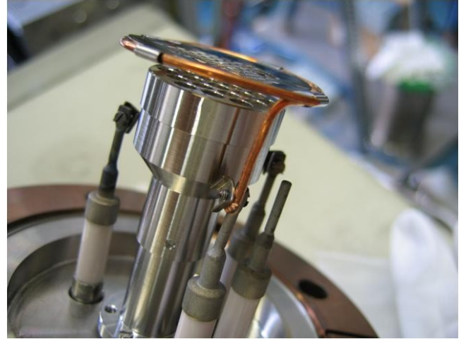
Fig. 9: Picture of a shielded pick-up equipped with a HV filtering grid.
