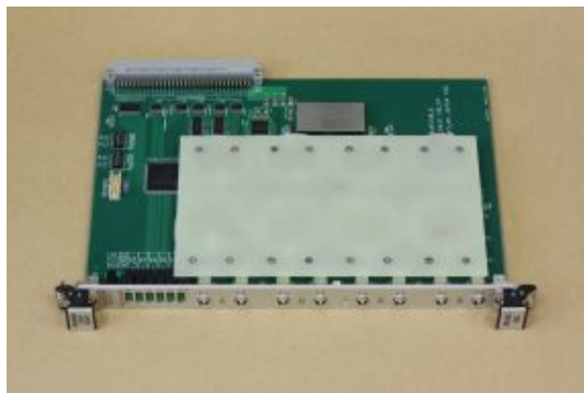
Figure 6: The delay module we have made to adjust the phase shift between the TGC and LHC bunch crossing signals. The circuit is housed in a VME 6 unit module
