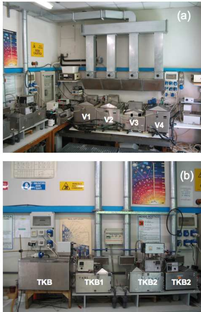
Figure 43: A view of the Bologna chemical etching Laboratory. (a) The V2 and V4 tanks are used for strong and soft etchings, the V3 tank for calibration purposes and the V1 tanks for the washing of the detectors after etching. (b) The TKB1 and TKB2 tanks, of smaller size, are used for the etching of a few detectors for calibration, TKB tank for pre-soaking, and TKB3 for their washing.
