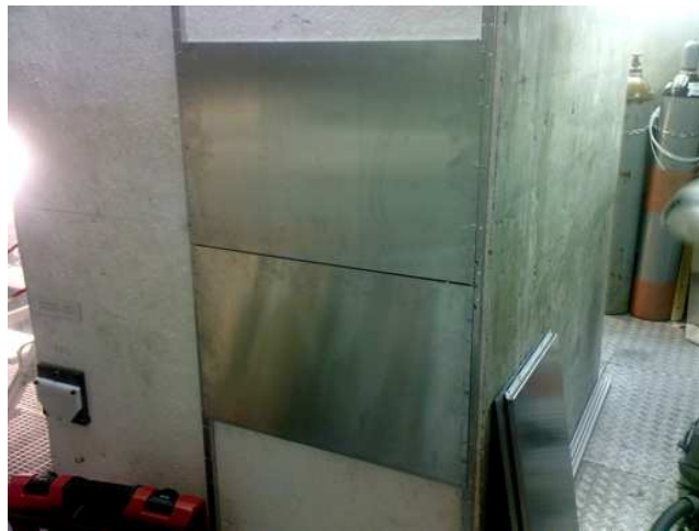
Figure 24: A test deployment of two MoEDAL aluminium housings each 50\text{ cm} \times 75\text{ cm} in area. The outer thickness of the housing is roughly 2 cm. Each housing will hold 6 basic MoEDAL NTD stacks and weight \sim 8 Kgs when fully loaded with detectors.
