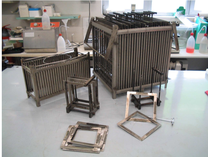
Figure 44: Stainless steel racks used for holding the CR 39 and Makrofol foils during etching. (a) Rack used for the etching of 25 \times 25 cm 2 plastic detectors in the V2 and V4 tanks. (b) in the V3 tank for calibration and (c) in the TKB1 and TKB2 tanks..
