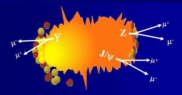
ATLAS performance in Pb+Pb collisions to measure quarkonium and Z via di-muon channel was studied by merging single J/ψ, Y and Z into Hijing Pb+Pb collisions at 5.5 TeV energy.
