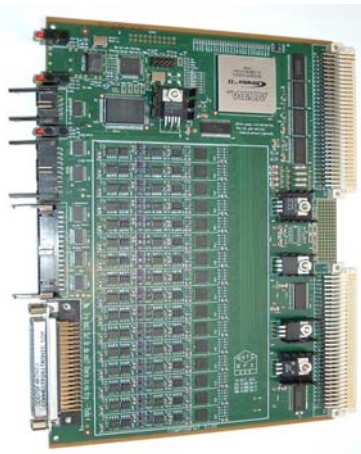
Figure 6: Prototype 14-Bit, 125 MHz ADC Module
