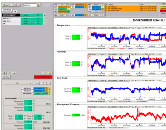
Figure 5: Ambient Environment panel in USA15 Level1
