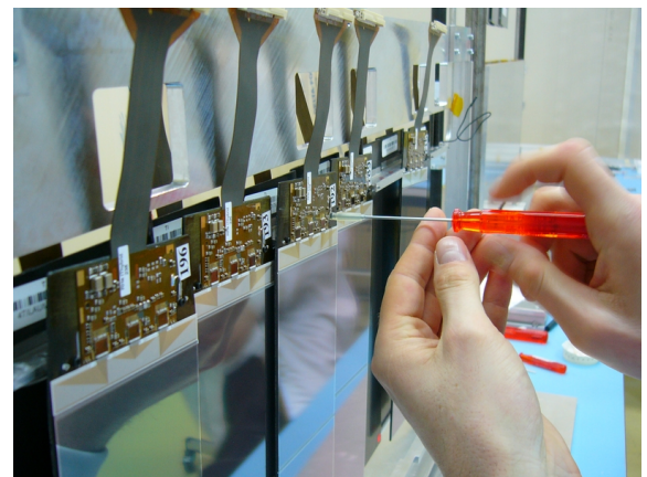
Figure 17 View of the fixing of the modules on the cooling rod, by starting with the backward modules and finishing with the forward modules.
