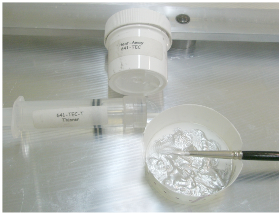
Figure 16 The thermal and electric conductive grease (left) is spread on the cooling rod (right) where the modules are intended to be fixed.
