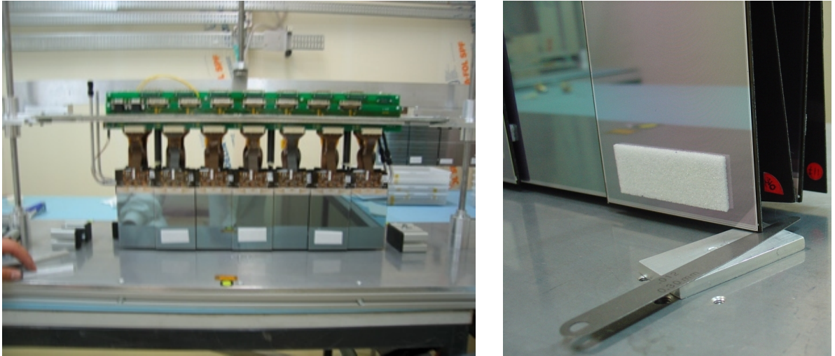
Figure 20 Resting on the dedicated stops, an assembly is ready for the test of the height of the sensor modules (left). On the right, one measures the distance, d , between the base plate and the bottom of the module supports, as shown on the drawing of Figure 19, using a calibrated wedge and precision blades.
