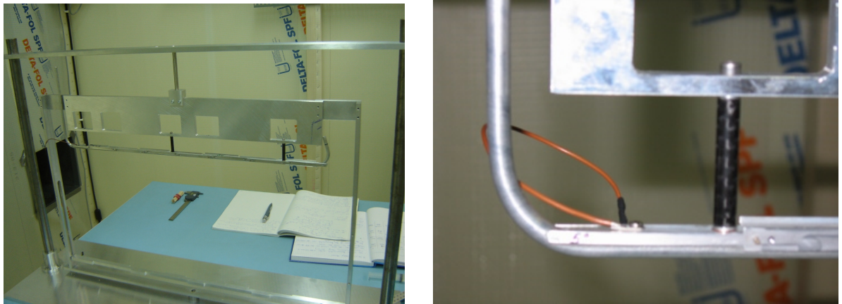
Figure 11 View of a cooling rod mounted on its support (left) with the help of the three colonnettes of 35 mm screwed on it (right). The thread for the grounding is also visible (right).
