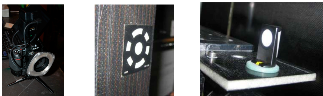
Figure 9 Camera, coded and non coded targets used for the photogrammetry measurements.
