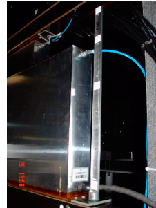
Figure 18 500mm-bars with four target stickers at 30,270,400 and 490mm.
