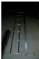
Figure 16 Weak positioning element (left) and the stiffer one that has replaced it(right).
